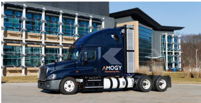
Fig. 3. Class 8 ammonia powered truck [2]
