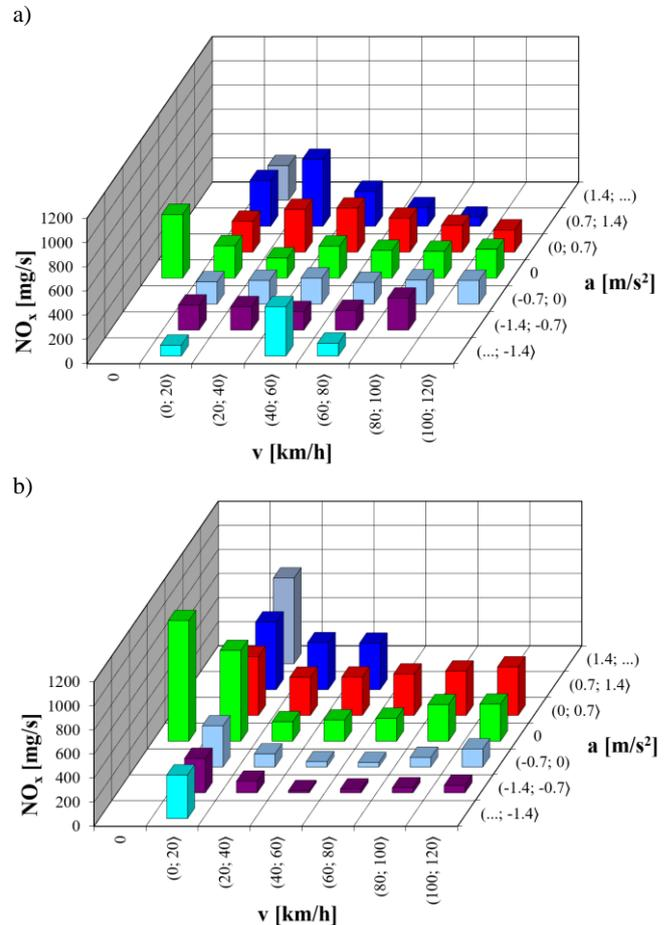
Fig. 11.  $\text{NO}_x$  emission intensity in speed and acceleration ranges: a) for research object A, b) for object B
