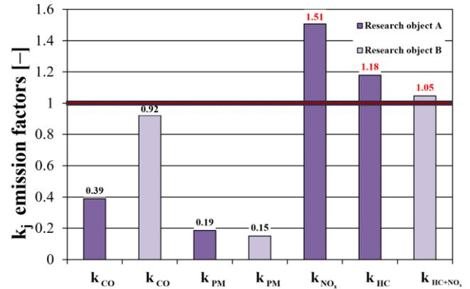
Fig. 15. The emission factor  $k_j$  for: CO, PM, NO<sub>x</sub> and HC
