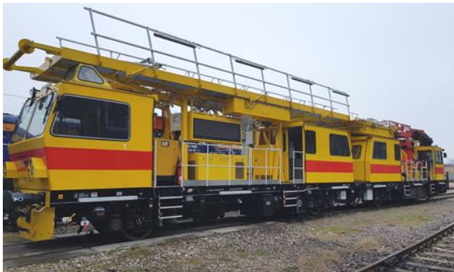
Fig. 4. General view of the PS-00.M/B type network train [19]
