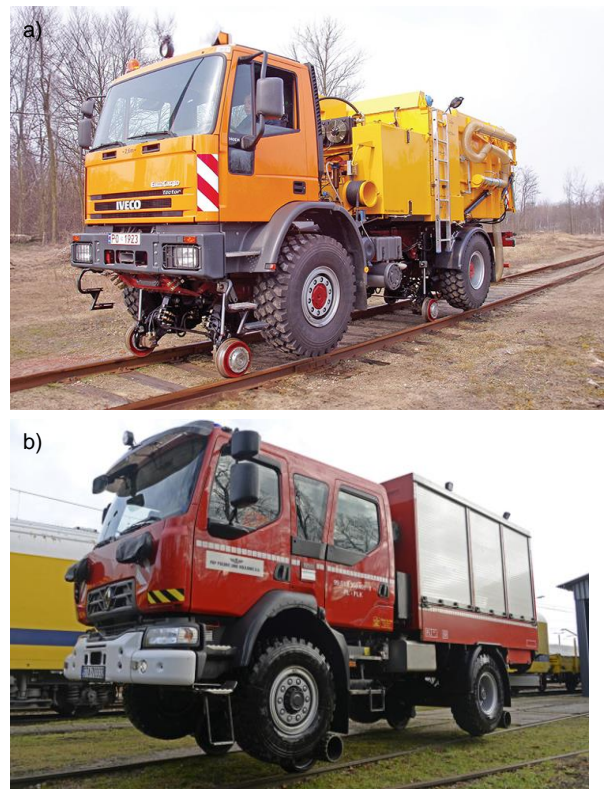
Fig. 6. Vehicle: a) rail-road vehicle for cleaning tram infrastructure [23], b) Technical Rescue rail-road Renault UniRoller-S [26]
