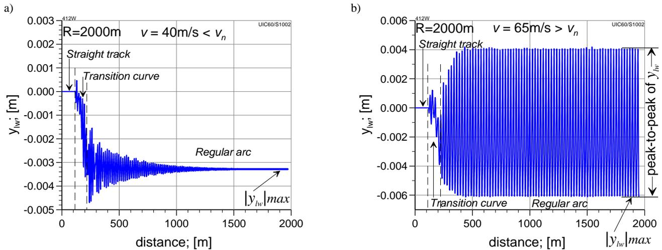
Fig. 3. The first wheelset lateral displacements  $y_{lw}$  versus distance: a) stable stationary solutions ( $40 \text{ m/s} < v_n$ ), b) stable periodic solutions (limit cycle,  $65 \text{ m/s} > v_n$ )
