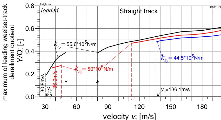
Fig. 8. The first wheelset derailment quotient  $Y/Q$  for different  $k_{zy}$  values:  $55.6 \cdot 10^5$  N/m (nominal value),  $50 \cdot 10^5$  N/m (90% of nominal value) and  $44.5 \cdot 10^5$  N/m (80% of nominal value)
