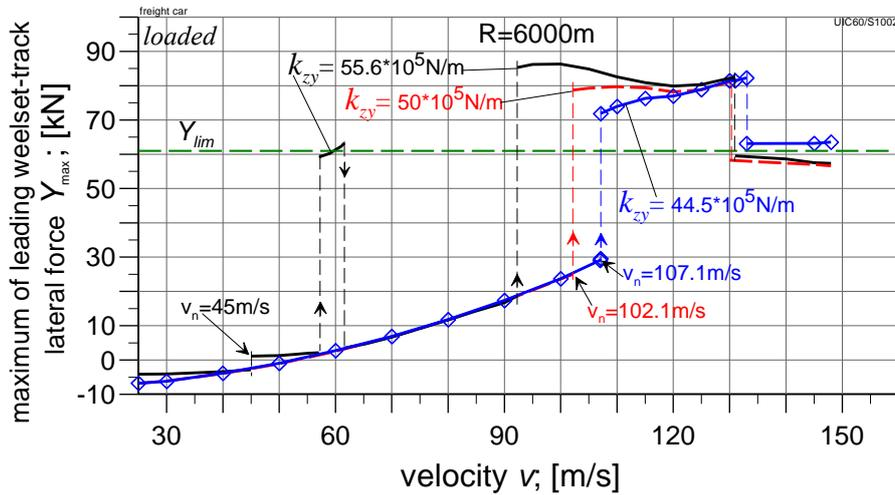
Fig. 10. The first wheelset-track lateral forces for different  $k_{zy}$  values:  $55.6 \cdot 10^5$  N/m (nominal value),  $50 \cdot 10^5$  N/m (90% of nominal value) and  $44.5 \cdot 10^5$  N/m (80% of nominal value). Curve track of curve radius  $R = 6000$  m
