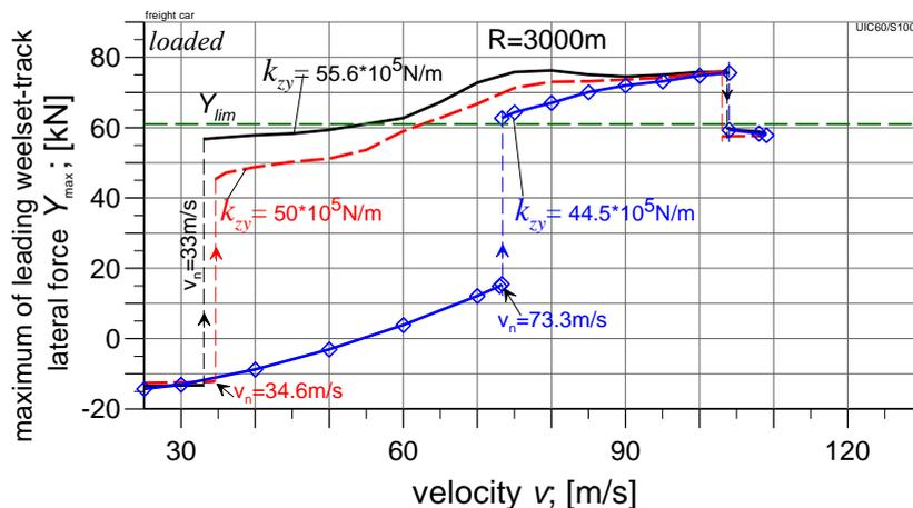
Fig. 13. The first wheelset-track lateral forces for different  $k_{zy}$  values:  $55.6 \cdot 10^5$  N/m (nominal value),  $50 \cdot 10^5$  N/m (90% of nominal value) and  $44.5 \cdot 10^5$  N/m (80% of nominal value). Curve track of curve radius  $R = 3000$  m
