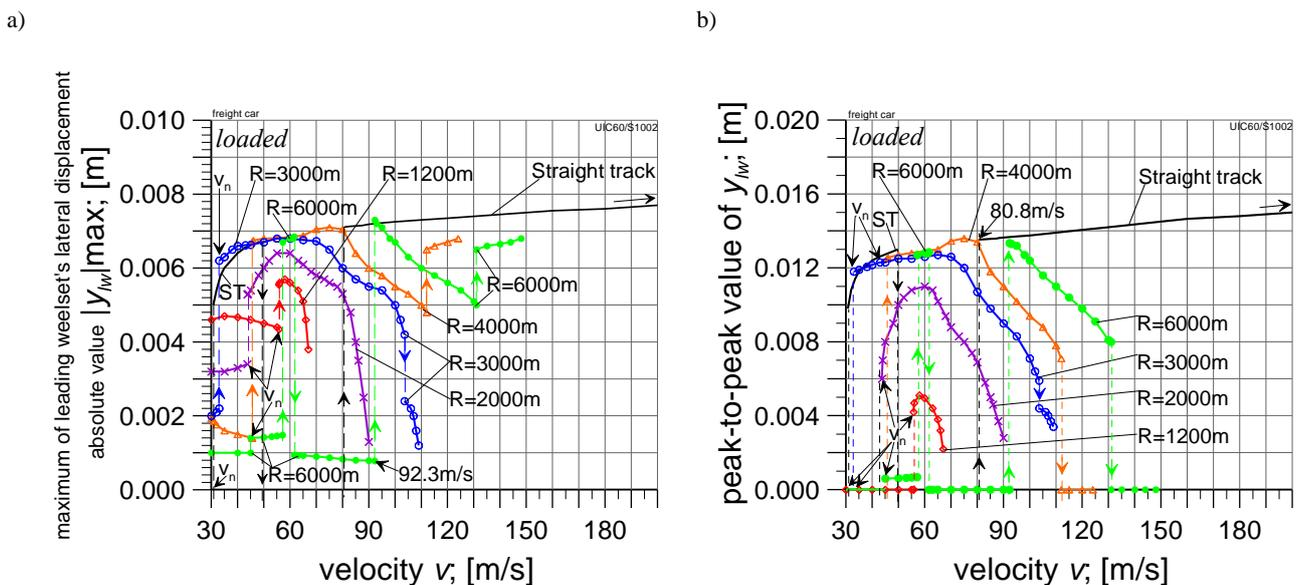
Fig. 5. The loaded vehicle model stability map: a) maximum of leading wheelset lateral displacements absolute value  $|y_{lw}|_{max}$  and b) peak-to-peak value of  $y_{lw}$  versus vehicle velocity
