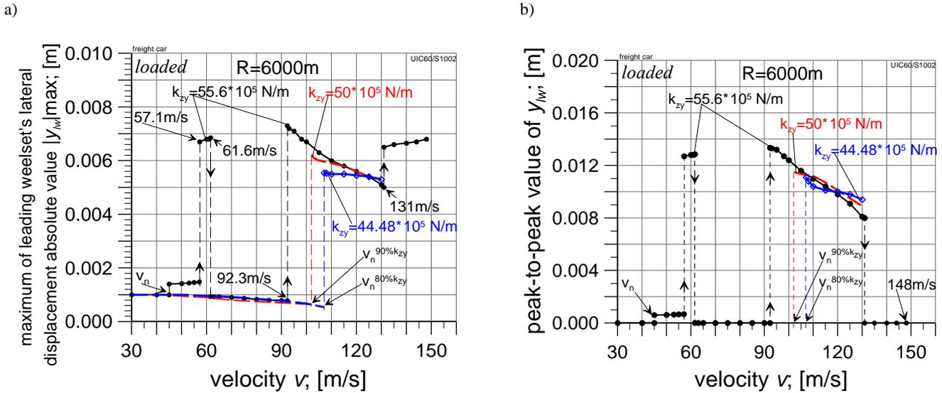
Fig. 9. Maximum of the first wheelset lateral displacements absolute value  $|y_{lw}|_{max}$  – a and peak-to-peak value of  $y_{lw}$  – b versus vehicle velocity for different  $k_{zy}$  values: nominal one ( $55.6 \cdot 10^5$  N/m), 90% of nominal value ( $50 \cdot 10^5$  N/m) and 80% of nominal value ( $44.5 \cdot 10^5$  N/m). Curved track motion of curve value  $R = 6000$  m
