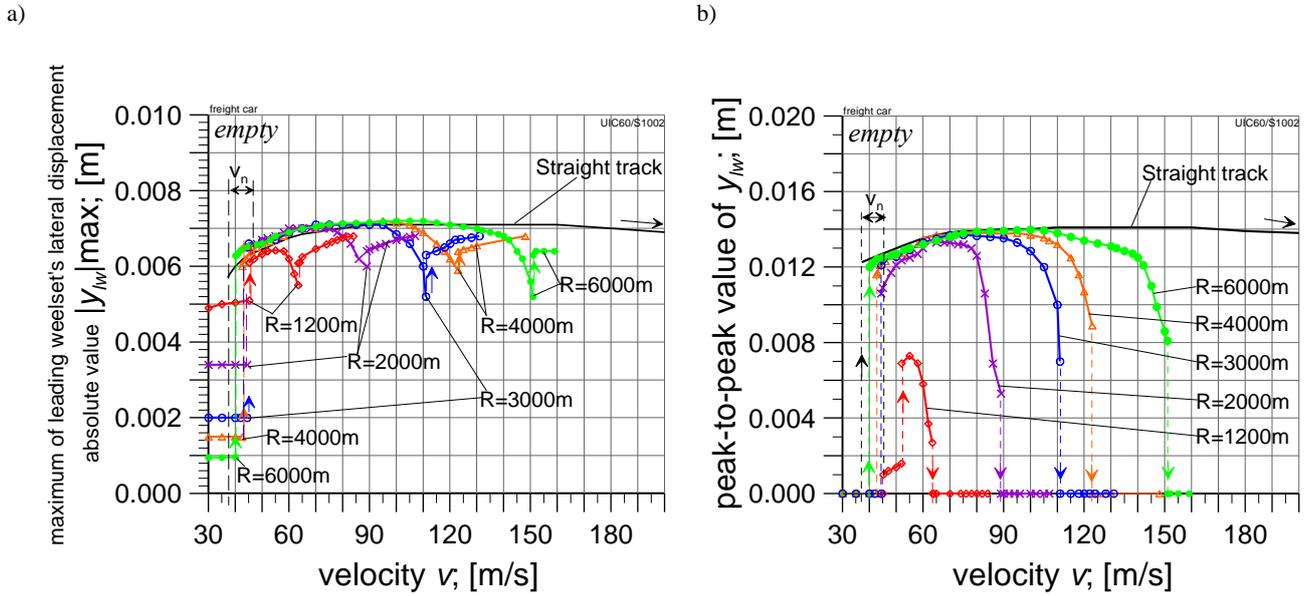
Fig. 4. The empty vehicle model stability map: a) maximum of leading wheelset lateral displacements absolute value  $|y_{lw}|_{max}$  and b) peak-to-peak value of  $y_{lw}$  versus vehicle velocity
