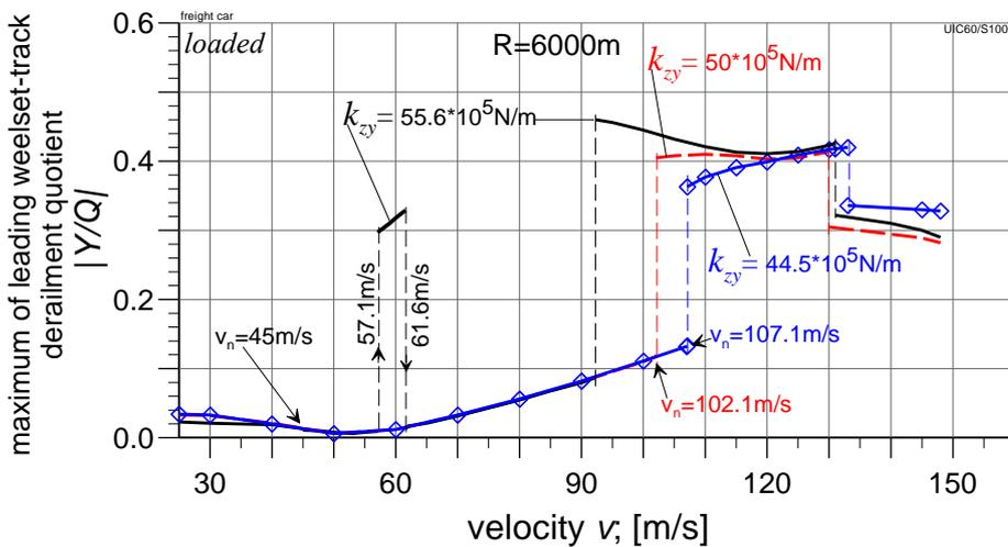
Fig. 11. The first wheelset derailment quotient absolute value  $|Y/Q|$  for different  $k_{zy}$  values:  $55.6 \cdot 10^5$  N/m (nominal value),  $50 \cdot 10^5$  N/m (90% of nominal value) and  $44.5 \cdot 10^5$  N/m (80% of nominal value). Curve track motion of curve radius  $R = 6000$  m
