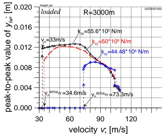
Fig.12. Maximum of the first wheelset lateral displacements absolute value  $|y_{lw}|_{\max}$  – a and peak-to-peak value of  $y_{lw}$  – b versus vehicle velocity for different  $k_{zy}$  values: nominal one ( $55.6 \cdot 10^5$  N/m), 90% of nominal value ( $50 \cdot 10^5$  N/m) and 80% of nominal value ( $44.5 \cdot 10^5$  N/m). Curved track motion of curve value  $R = 3000$  m
