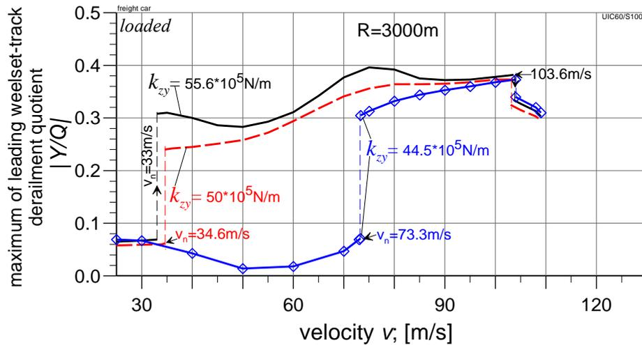
Fig. 14. The first wheelset derailment quotient absolute value  $|Y/Q|$  for different  $k_{zy}$  values:  $55.6 \cdot 10^5$  N/m (nominal value),  $50 \cdot 10^5$  N/m (90% of nominal value) and  $44.5 \cdot 10^5$  N/m (80% of nominal value). Curve track motion of curve radius  $R = 3000$  m
