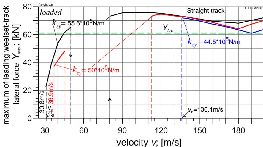
Fig. 7. The first wheelset-track lateral forces for different  $k_{zy}$  values:  $55.6 \cdot 10^5$  N/m (nominal value),  $50 \cdot 10^5$  N/m (90% of nominal value) and  $44.5 \cdot 10^5$  N/m (80% of nominal value). Straight track motion
