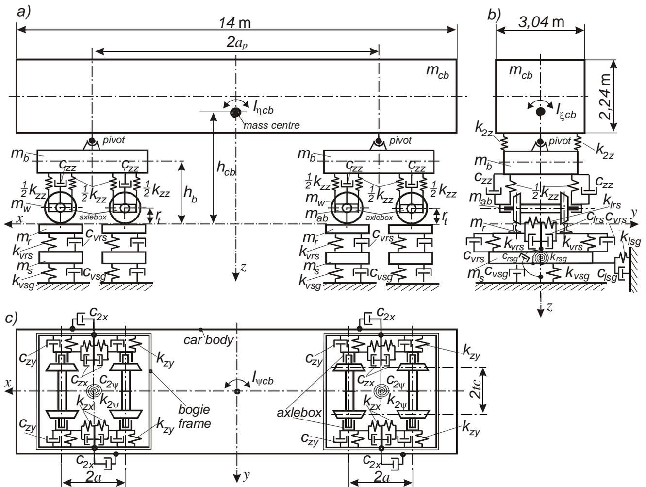
Fig. 2. Diagram of the freight vehicle – track system: a) side view, b) front view, c) top view
