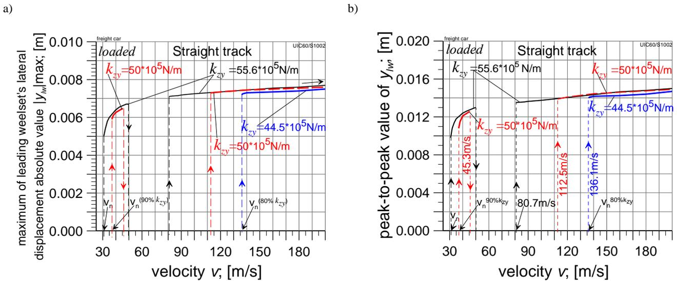
Fig. 6. Maximum of the first wheelset lateral displacements absolute value  $|y_{lw}|_{max}$  – a and peak-to-peak value of  $y_{lw}$  – b versus vehicle velocity for different  $k_{zy}$  values: nominal one ( $55.6 \cdot 10^5$  N/m), 90% of nominal value ( $50 \cdot 10^5$  N/m) and 80% of nominal value ( $44.5 \cdot 10^5$  N/m). Straight track motion
