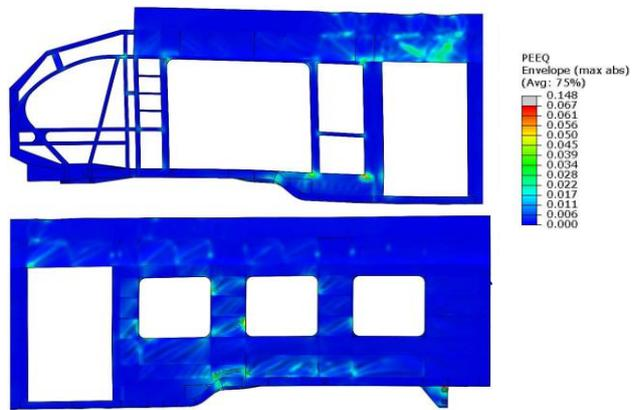
Fig. 16. Plastic deformation of the leading vehicle structure – side view
