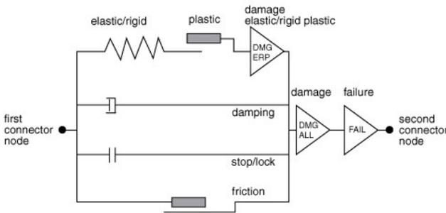
Fig. 6. Diagram of a connector type element
