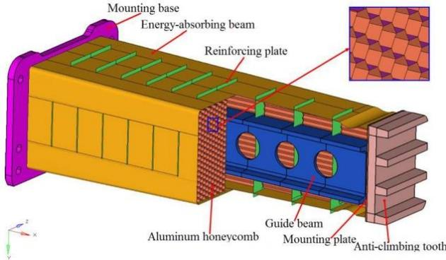
Fig. 5. The partial cross-sectional view of the example of anti-climbing device [5]
