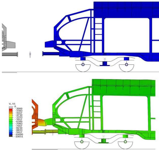
Fig. 12. The edge section of the lead vehicle at the beginning and end of the simulation (V1 – longitudinal velocity in the X axis)
