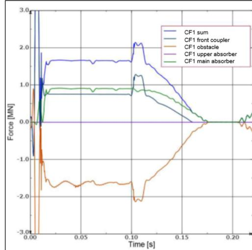
Fig. 15. Longitudinal components of the contact forces between the front end wall
