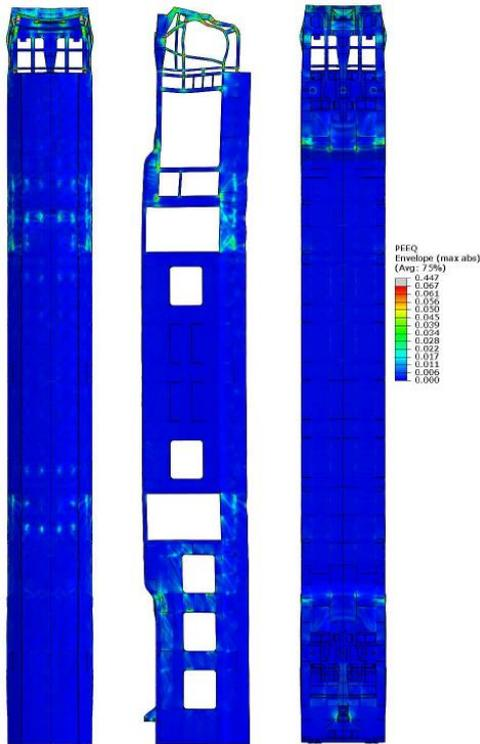
Fig. 23. Plastic deformation of the leading vehicle structure
