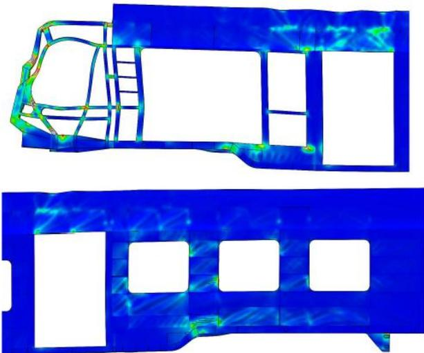
Fig. 24. Plastic deformation of the leading vehicle structure – side view
