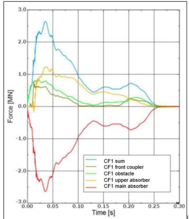
Fig. 20. Longitudinal components of contact forces between the front face of the evaluated vehicle and the flexible obstacle (180 Hz filter)
