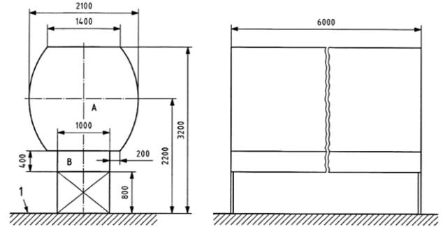
Fig. 8. Level crossing 15 t deformable obstacle
