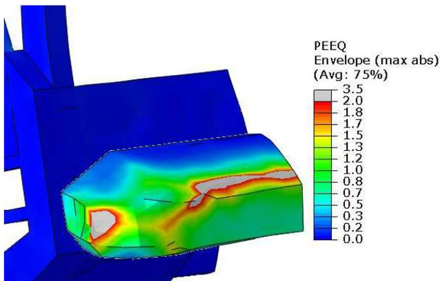
Fig. 19. Deformation of the honeycomb top absorber
