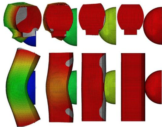
Fig. 10. Displacement stratification in successive stages of the obstacle verification test
