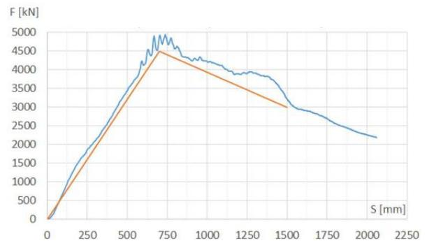
Fig. 9. Characteristics of the deformable obstacle – reference and obtained in simulation
