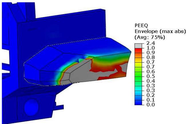
Fig. 13. Deformation of the honeycomb top absorber
