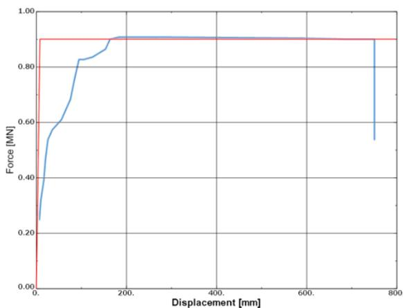
Fig. 7. Force-displacement curve (blue line – research, red line – simulation)
