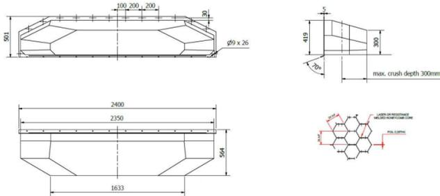
Fig. 2. Honeycomb main absorber
